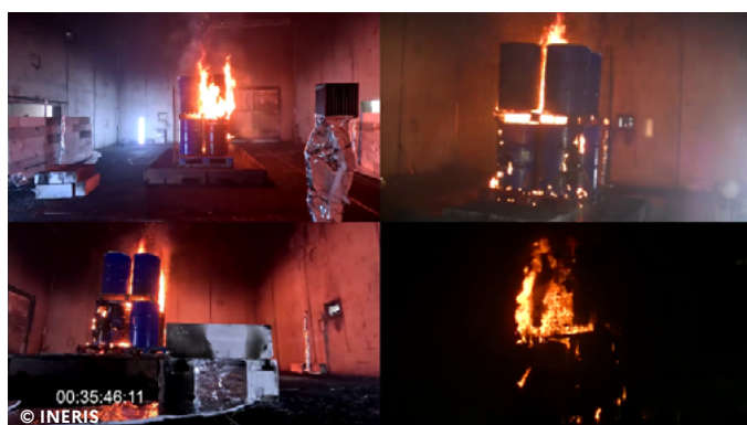
Propagation tests on storage drums
