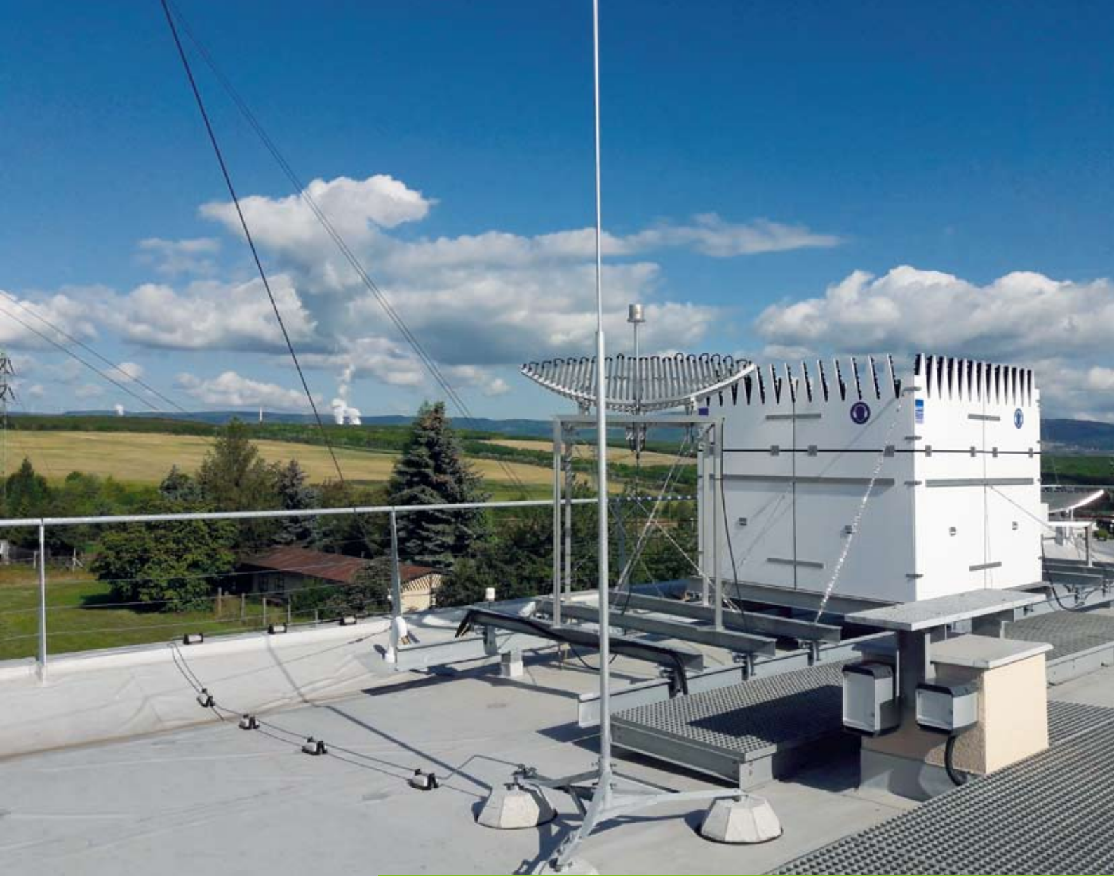
▲ The Radioacoustic system (Doppler SODAR – Sonic Detection And Ranging) for atmospheric boundary layer monitoring at Tušimice Observatory.
