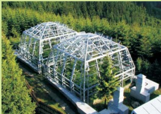
Glass domes with adjustable windows used for the simulation of elevated CO 2 concentration in the atmosphere (Bílý Kříž, Beskydy Mts.).
