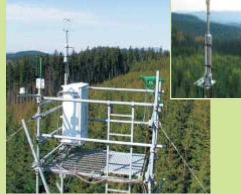
Eddy-covariance system for the measurement of energy and substances fluxes between the boundary layer of the atmosphere and the ecosystem.
